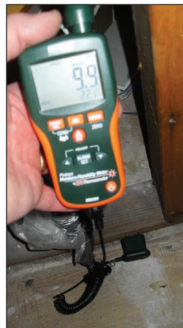
Figure 5: Use of a penetrating (pin-type) moisture meter to verify that wood frame has a water content of less than 15 percent
