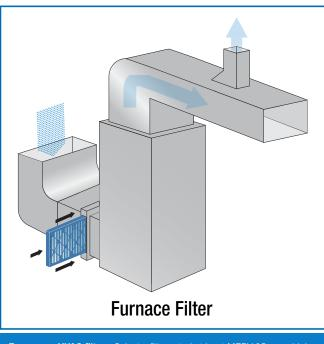
**Furnace or HVAC filter**—Select a filter rated at least MERV 13 or as high as your system will accommodate.
