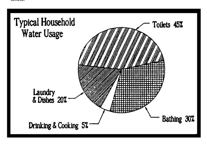
Even using a toilet dam or putting a container filled with rocks in the toilet tank can reduce water use by 25 percent.
