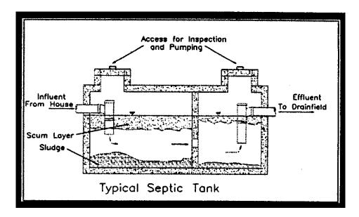
This can happen on days when water use is unusually high (laundry day, for example), or more often if the septic tank is too small for the needs of the household. Some septic tanks are outfitted with a baffle screen. This screen serves to protect the drain field from receiving solids.
