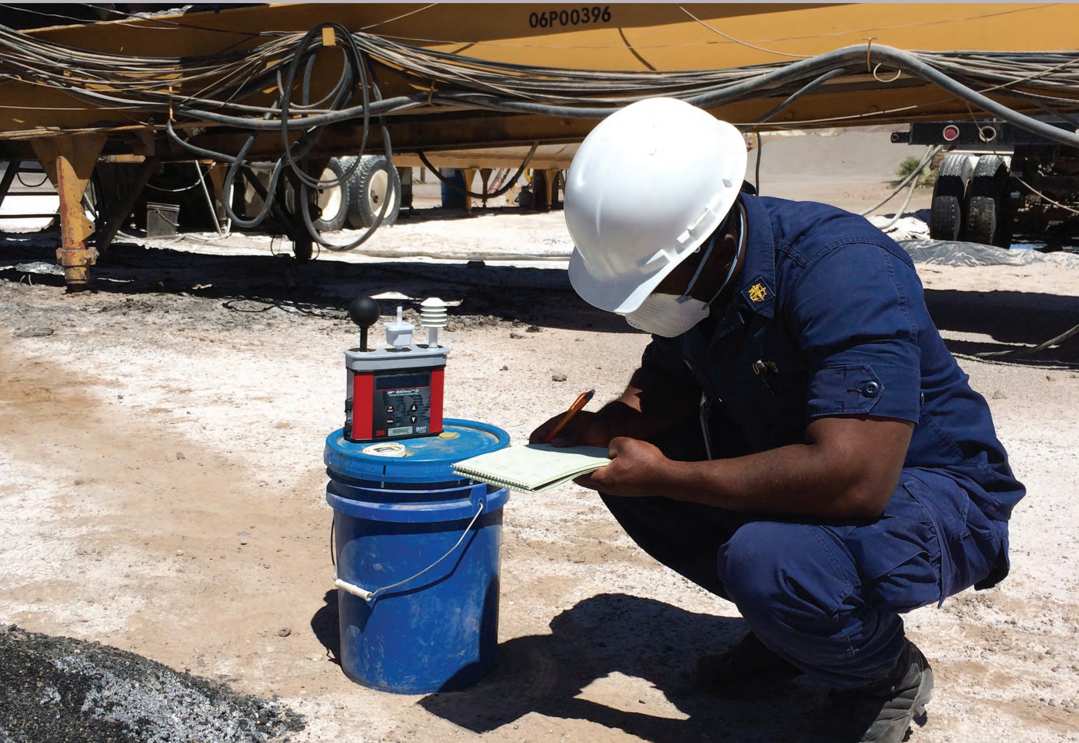
LT Ampadu recording measurements from a wet bulb globe thermometer as part of a follow-up indoor air quality investigation.
