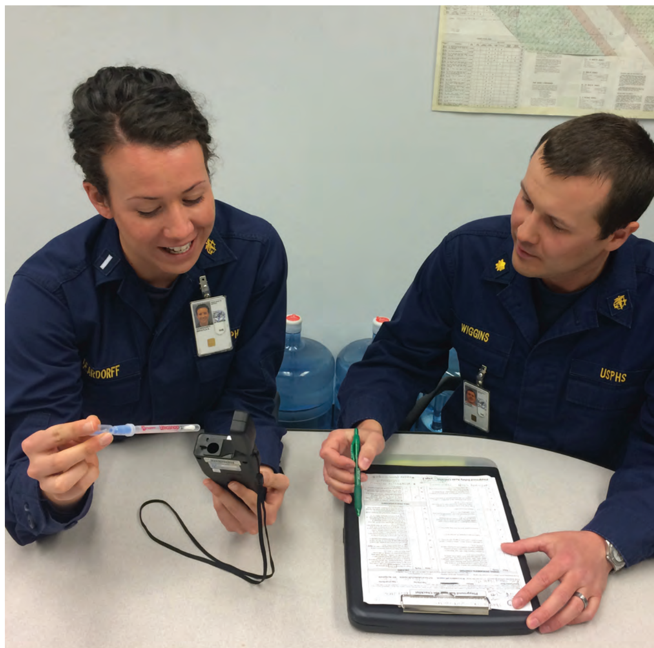
LTJG Deardorff and LCDR Wiggins use adenosine triphosphate bioluminescence to assess the effectiveness of surface disinfection in a clinic.
