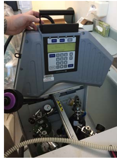
The MIRAN SapphIRe was used to detect a leak in a portable nitrous oxide system.
