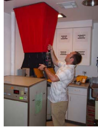
Measuring ventilation air flows at the Stockbridge-Munsee Health Clinic.
