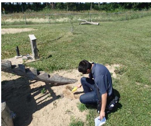
Assessing the depth of sand for fall shock protection at a playground.
