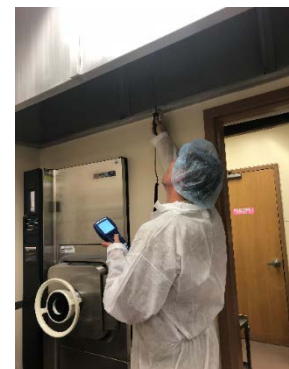
CAPT Brian Hroch using a TSI air velocity meter, Santa Fe, NM
