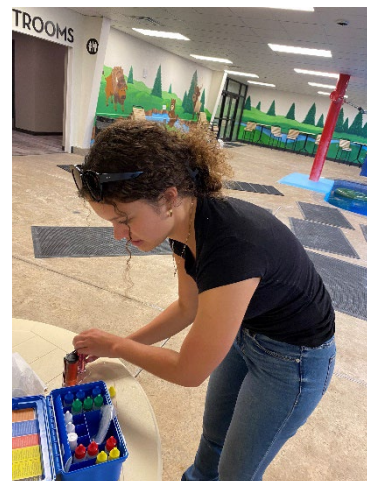
Measuring the water chemistry of a hotel swimming pool
