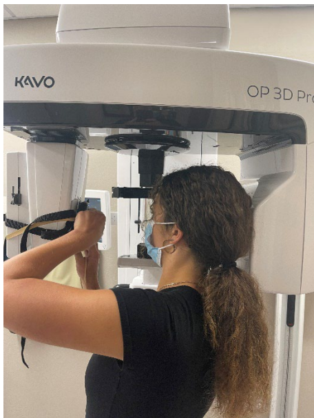
Using an x-ray meter to monitor exposure to radiation from a dental panoramic x-ray machine
