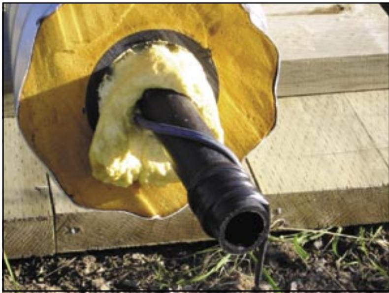
**Figure 35:** Cross-section of Arctic pipe used for Alaska construction projects.
