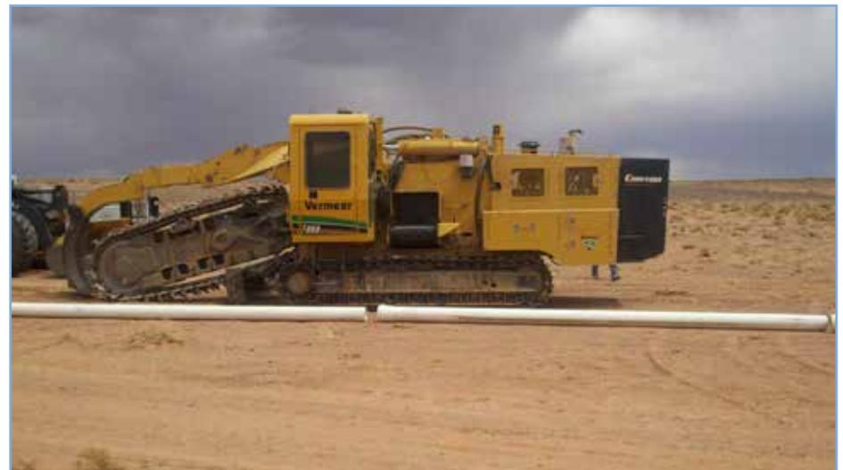
Vermeer trencher used to lay PVC pipe.
