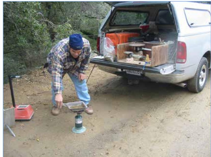
Checking the compaction of soils during construction, California.
