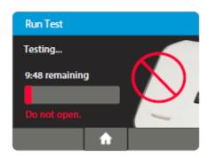
Caution: This screen will be displayed for up to 30 seconds once the Transfer Cartridge is detected. If the instrument does not detect that the lid has been closed by then, it will time out and all test pieces (Sample Receiver, Test Base, and Transfer Cartridge) must be removed and discarded. The instrument will proceed to the Home screen. Collect a new sample from the patient. Press Run Test and restart the test using a new Test Base and Sample Receiver.
