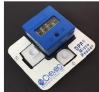
DPP Micro Reader with Test Device Holder and Test Device
