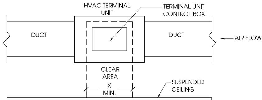
2 HVAC TERMINAL UNIT ELEVATION
