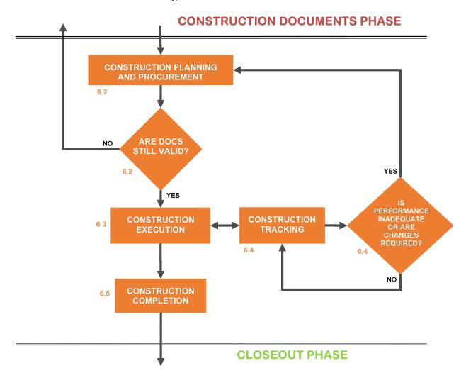
**Figure 6.1 Construction Phase**
