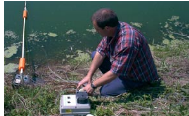
Figure 26: Contractor completing sampling and analysis of lagoon effluent.
