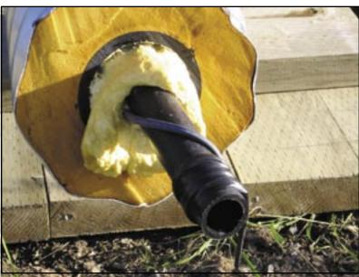
**Figure 35:** Cross-section of Arctic pipe used for Alaska construction projects.
