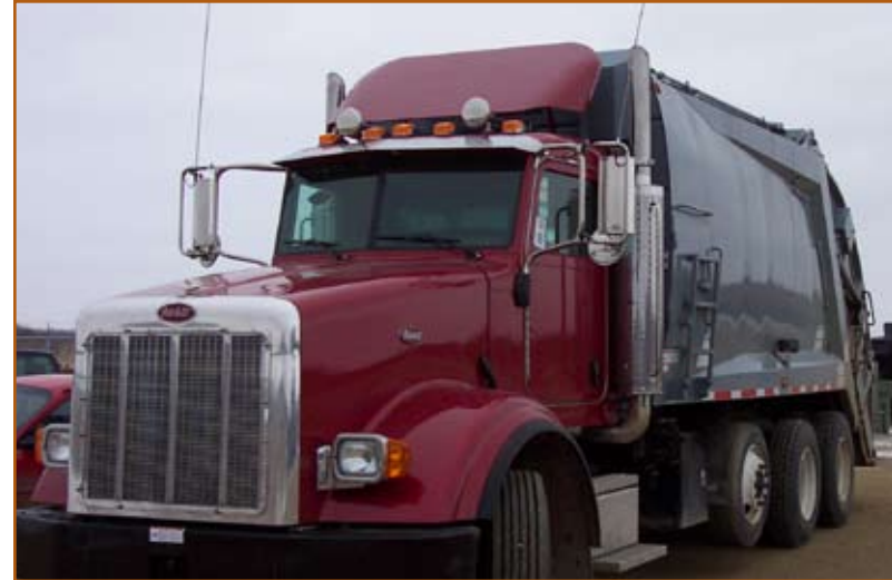
Figure 24: Twenty-five cubic yard, rear load compactor truck purchased for Spirit Lake Tribe Solid Waste Program.
