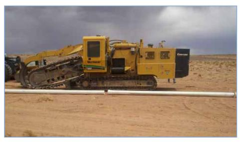
Vermeer trencher used to lay PVC pipe.
